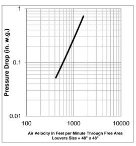
The AMCA Certified Ratings Seal applies to Air Capacities in the intake model only Data corrected to standard air density Tested to AMCA 500-L, Figure 5.6
